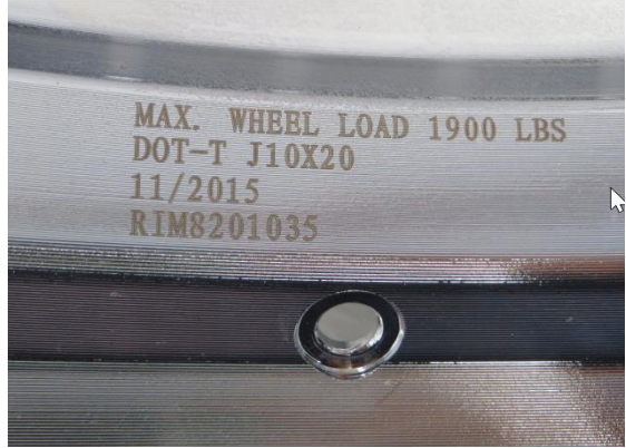
Laser Engraving on inner rear part of barrel
